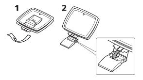
Connect the loop antenna's wires to the AM antenna terminals.
